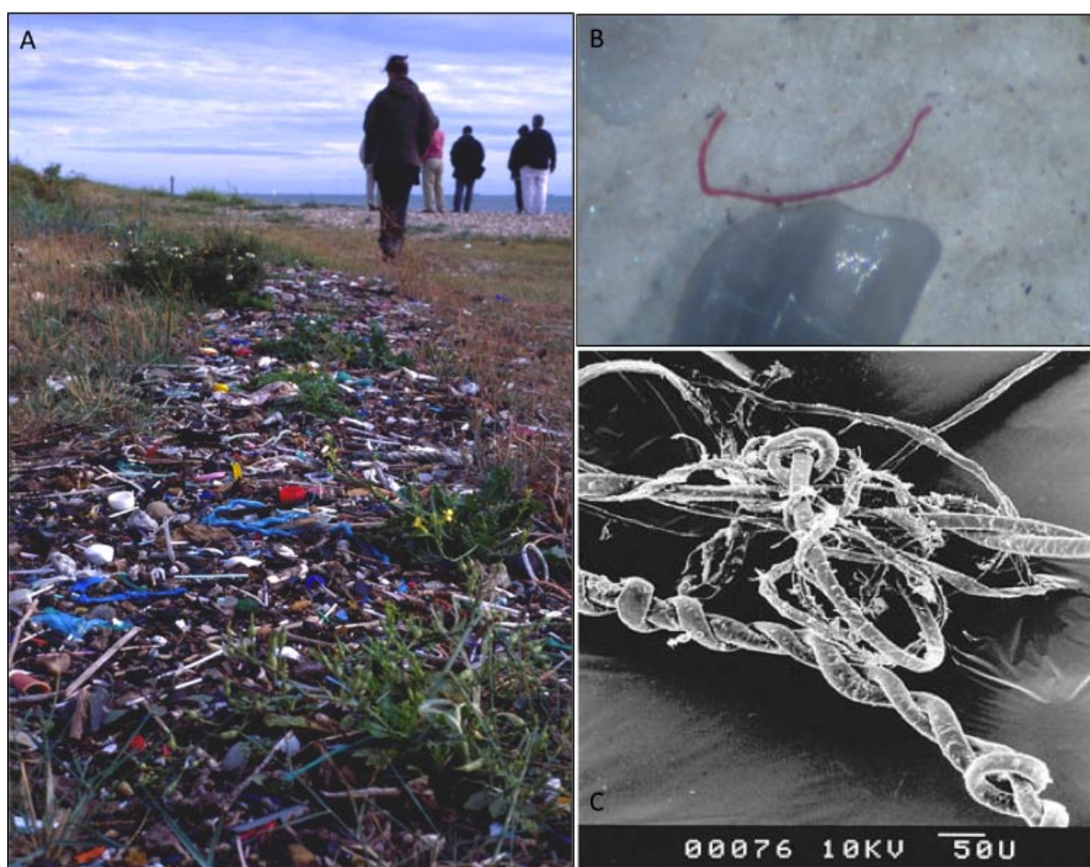
Figure 1: A) Marine debris on a strandline where it fragments into smaller pieces. B) A fragment of microplastics next to a grain of sand found on a beach in Cornwall, UK. C) Scanning electron microscope image of microplastic fragments. Source: R.C. Thompson.
